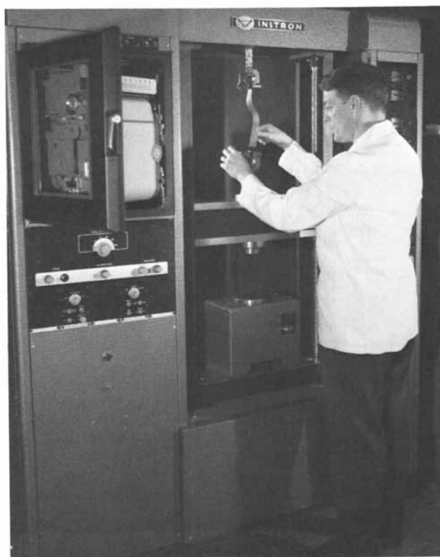
Figure 2. Tensile strength measurement with the Instron Universal Testing machine
